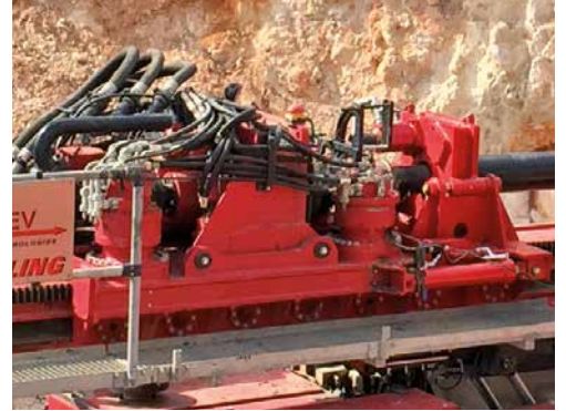
Robust double rotary head with torque of 20 kNm - 90 kNm
