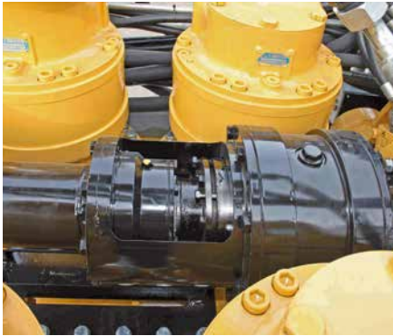
Mud swivel on tapered roller bearing
