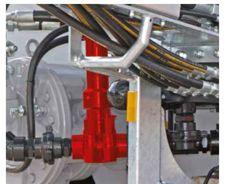
Bentonite supply, hydraulically lockable with by-pass
